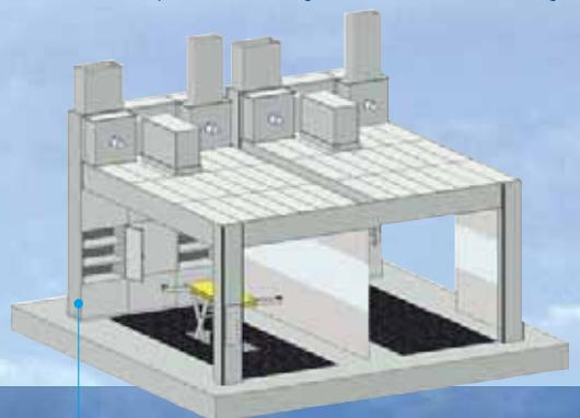
Air replenishing system with stacked unit and hot water heating coil
